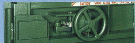
Patented front geared wheel lock is standard on several models.
